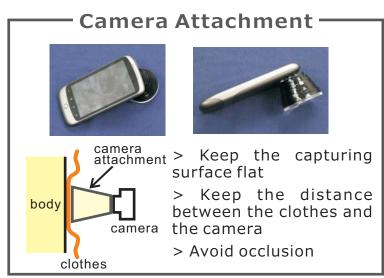
We encode a position information pattern on fabric. A camera captures the pattern and detects its own position and orientation on the fabric.
